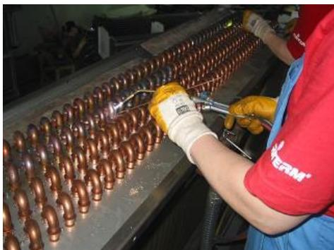
All copper tube-curve, copper tube-collector connections, connections used in frames and all connections of fittings should be done with the "Brazing" method and the solder wires used for soldering should be silver alloy solder wires.
