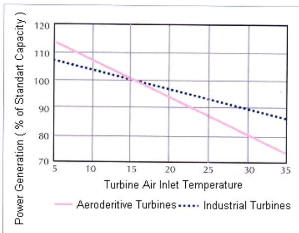
When compared to standard capacities in conditions where ambient temperature is above 15°C, the prevention or reduction in gas turbine power losses can be viewed as the primary benefit of Turbine inlet air cooling. Cooling the combustion turbine inlet air below 15°C also enables power plant owners to obtain a power output above the standard generation capacity of the gas turbine.
