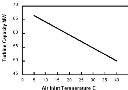
FIGURE:2 Effect of Air Inlet Temperature on Capacity for the 7B Combustion Turbine, NEBRASKA
