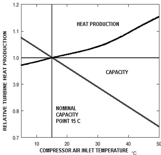
The variation curve of the combustion turbine capacity and heat generation as a function of air inlet temperature has been given in Figure 1. Energy capacity measurement values versus air inlet temperature for a GE Frame 7B combustion turbine installed in Lincoln, Nebraska have been given in Figure 2.
