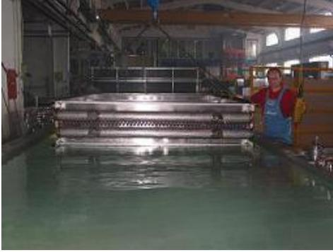
The Cooling Coil should be subjected to an imperviousness test under 20 kg/cm<sup>2</sup> of pressure.
