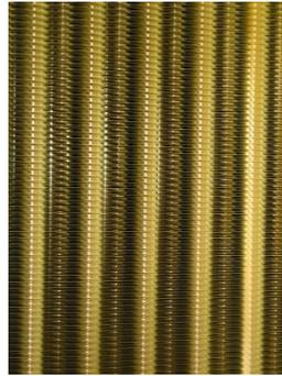
Fin Press Lines and fins processes according to mould, form and spacing. Tight contact achieved between tubes with the Arrangement and Blowing process. Main finned block
