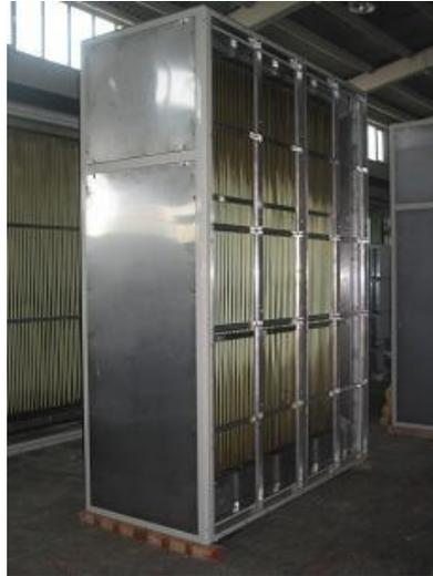
Figure: 13.1-2-3 View of the Cooling Unit Cell from the Drop Eliminator and the Filter sides (Filter cartridges are installed on location).
