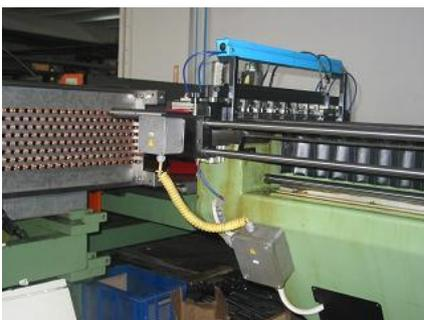
**In consideration of performance and cost-friendliness, the most appropriate tubing material for cooling coils is copper.** For this reason, the copper tubes used must be manufactured per international standards. The most important parameter in applications is the wall thickness of the tube. The recommended tube and curve wall thickness is the range 0.635 mm – 1.00 mm
