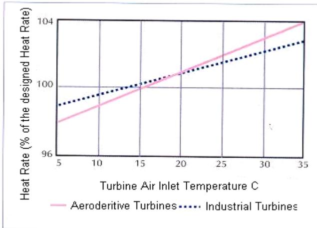
An increase in air inlet temperature of 15°C to 38°C increases the heat ratio. This leads to an approximate 4% drop in fuel efficiency. The drop in fuel efficiency can be prevented by cooling the combustion turbine inlet air. For a typical gas combustion turbine, cooling the inlet air from 15°C to 6°C lowers the heat ratio and increases fuel efficiency by approximately 2%.
